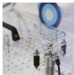
Basket on pneumatic cylinder for non destructive immersion test
